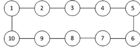
Fig. 2. Topological structure of the circular network with 10 nodes.
